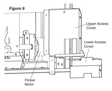
**A** CAUTION: When removing and replacing the flicker motor try to keep any slight bending of the flicker rod minimal so as to not damage it. If flicker rod is damaged, it should be replaced to ensure proper operation.
