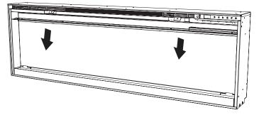
middle, along the top of the opening, ensuring that neither the bracket nor the partially reflective glass falls out of the unit. (Figure 5)
