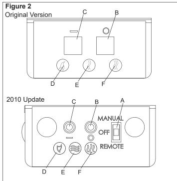
Level 1 - Flame effect only, twice activates Level 2 -Flame effect and Purifire<sup>™</sup>, three times activates Level 3 - Flame effect, Purifire<sup>™</sup> and heat.
