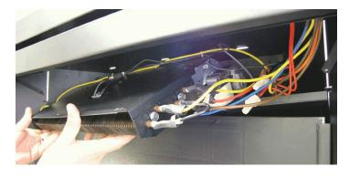
Interior Bottom View of Voltage Selector Switch and Over Temperature Light
