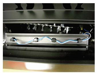
Manual Controls with Remote Control Bracket Removed
