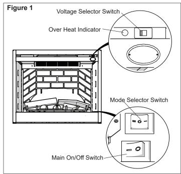
Main Power Switch - Energizes firebox and flame.
