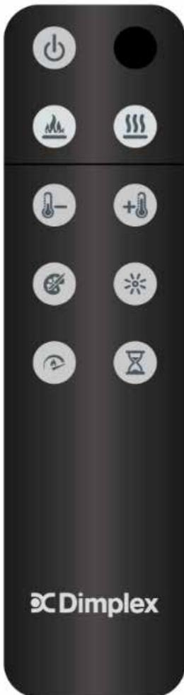
The multi-function IR (infrared) remote control has a range of approximately 20 ft (6 m). To operate, the remote control must be pointed toward the front of the electric fireplace.
