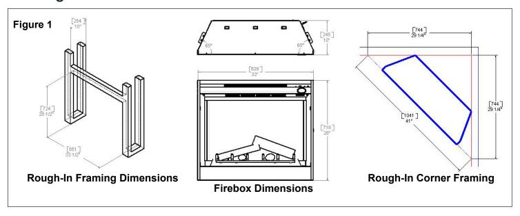
This fireplace is a zero clearance design. No combustibles can be placed on the top surface of the fireplace. Combustibles may be installed to the edge of the unit. Four mounting flanges on the sides of the unit are provided to facilitate installation. Insulation and vapor barrier should be placed a minimum of 2" (5.1 cm) from the unit.
