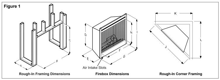
This fireplace is a zero clearance design, with the exception of the top of the unit, where any insulation and vapor barrier should be placed a minimum of 2" (5.1 cm) from the unit. No combustibles can be placed on the top surface of the fireplace.
