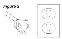
♠ DANGER: Improper connection of the equipment-grounding conductor can result in a risk of electric shock. Check with a qualified electrician or serviceman if you are in doubt as to whether the product is properly grounded.
